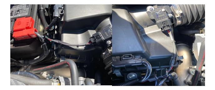
The one branch with two connectors mounts INLINE to the Mass Airflow Sensor (MAF). Route it to that general area, disconnect your MAF, and plug that factory connector into the male connector on the harness. Connect the other one to the MAF.
