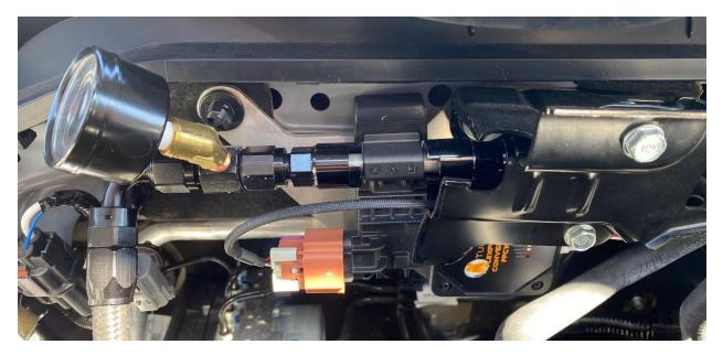
Install the 5/16" SAE Fuel Line Adapter to 6an male to the factory hardline. Next use the 6an Swivel coupler to connect between the 3/8" SAE fitting on the Flex Sensor and connect them together. You can leave all of the fittings slightly loose as you install everything, and then go back and tighten each fitting later.
