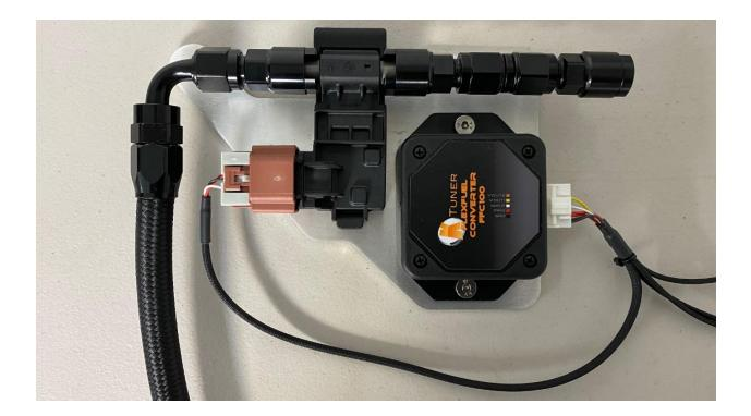
\*\*\* IMPORTANT \*\*\* Next take the 5/16 SAE quick disconnect (with plastic) and install that into the 45 degree hose end and tighten. It will be difficult to tighten later if you do not do it before connecting it to the HPFP (high pressure fuel pump)
