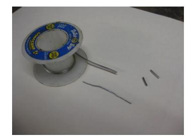
Clay and playdough are a messy waste of time because you can't measure it accurately and it often sticks to valves and tears. It is handy for making impressions of shapes inside the chamber that we can never see, but solder definitely does a better job on P2H clearance in my opinion.
