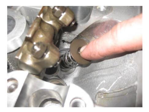
Now we've got to bolt the degree kit onto the head. Here is my old Swiss cheese prototype mocked up on the windowed dummy head without indicators, because it's easier to install without them mounted to the beam.
