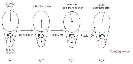
simple illustration to help understand the 2:1 ratio between crank and cam, as well as the difference between advancing and retarding the camshaft timing. note the red dots that always stay in sync, only the camshaft itself changes position relative to the crank, never the cam gear.
