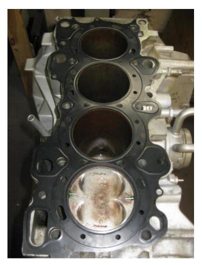
Keep in mind the images here are just mocked up parts I had laying around for reference. Start with a block and crank, with at least one piston/ring set installed. I prefer to use only one intake and one exhaust valve for all clearancing work. It's tedious, but a race motor is assembled, torn down, modified and reassembled numerous times before final building.
