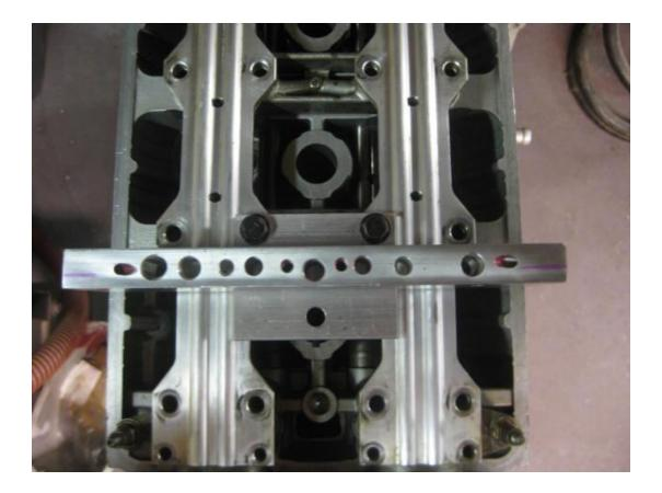
Note the orientation of this kit. The magic marker lines represent the offset holes that all current kits have. They are to be oriented closest to the cam gears, and are to offer the dial indicators some extra clearance for swinging over to either valve.
