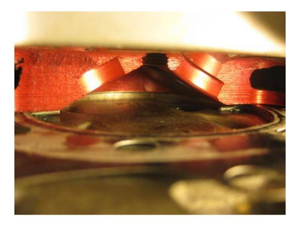
Remove cylinder head and measure solder at the thinnest point. If there is no definite flattening of the solder, you chose a solder that was too thin. Pull the head back off and start over with thicker solder. Is this getting tedious yet?
